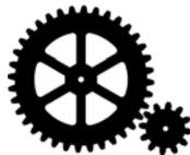
$$\frac{\text{Turns of output gear} \rightarrow T_o}{\text{Turns of input gear} \rightarrow T_i} = \frac{N_i}{N_o}$$
